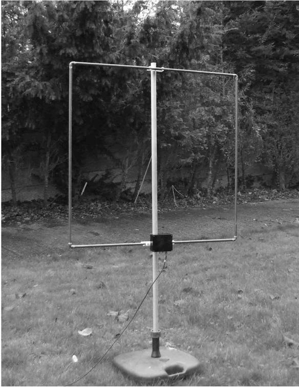
Figure 1 – 1m<sup>2</sup> bandpass loop antenna
