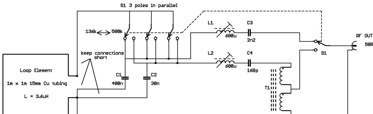
Figure 3 Band-switched  $136\text{kHz}/500\text{kHz}$  loop
