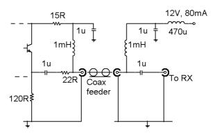
Figure 5 – Remote DC feed to preamp
