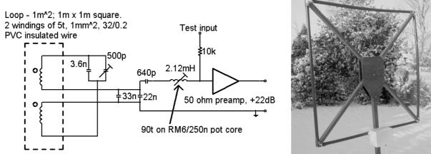
Figure 1 – 1m<sup>2</sup> bandpass loop
