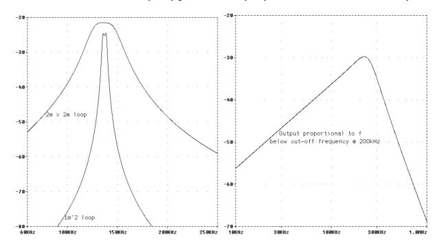
Figure 6 – Simulated frequency response of the loop antennas
