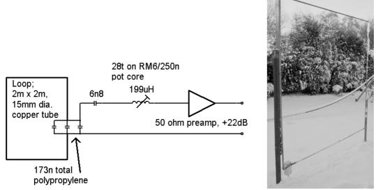
Figure 2 – 2m x 2m Bandpass Loop
